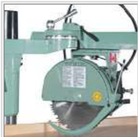
Pivot axis always at point zero
