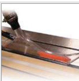
See-through blade guard with splitter and anti-kickback pawls
